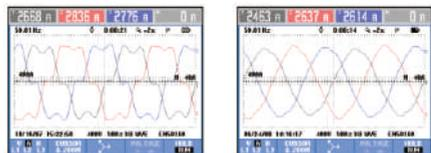
Waveforms and RMS values of phase currents before and after IPS AHFs were installed
