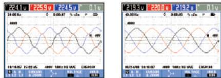
Waveforms and RMS values of phase voltages before and after IPS AHFs were installed
